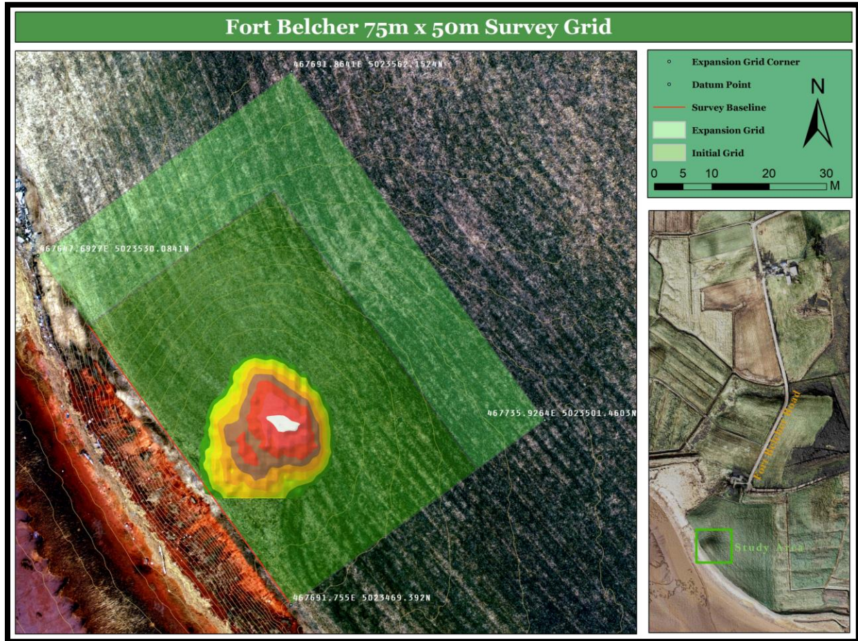
Figure 10: Geophysical survey grid showing the originally surveyed baseline, original grid and expansion grid. A LiDAR derived DEM is overlaid at the top of the hill, thought to be the height of land that Fort Belcher once stood, as noted in Figure 4.
