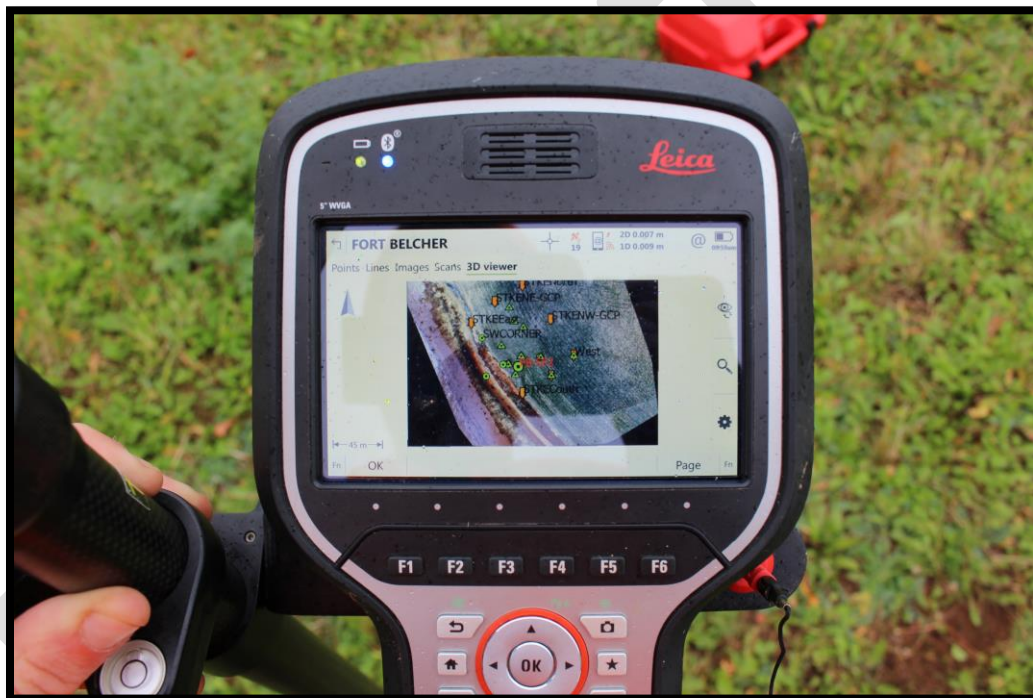
Figure 9: Screen of the Leica GSI4 Smart Antenna RTK GNSS data collector while staking out shovel test locations at Fort Belcher.
